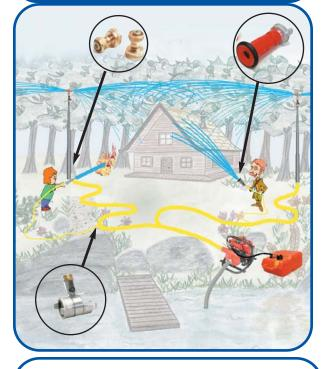
Kit "D" provides for a full application with sprinkler protection and dual Hose Nozzle connections, as depicted in the above sketch. (Sprinkler poles not included in the kit, however can be made available, at extra cost, through our installation program).
